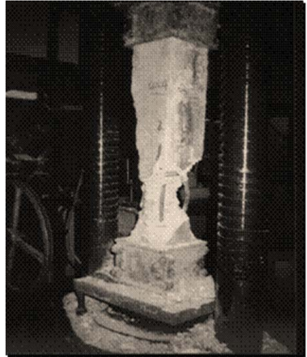
Fig. 4 : Typical crushing failure mode of columns
