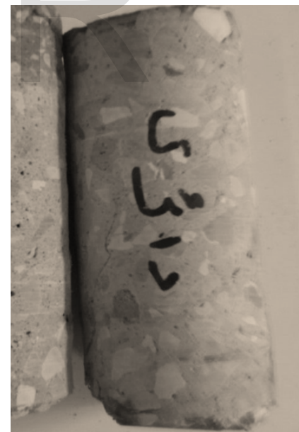
Fig. 5 : Core specimen cut from a circular column
